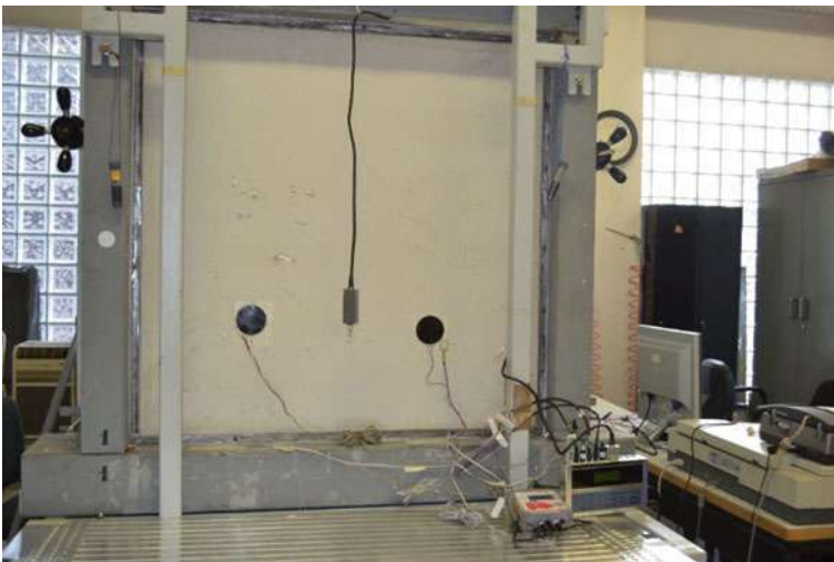
Fig. 3 Sample view in front of the climatic chamber and sensor wiring
