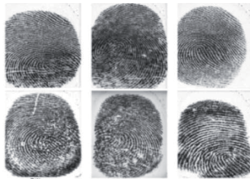
Figure 4. Fingerprint examples from LivDet2009 database [14], real cases (top line), and fake cases (bottom line).
